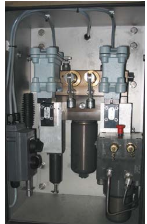
Shown with remote control 0, Line Break Control 1h and Torque Limit Device D
