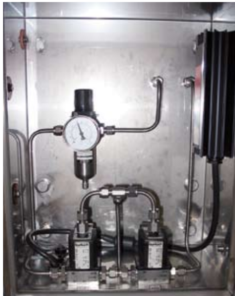
Control type K shown with two solenoid valves (one ESD) and heating unit
