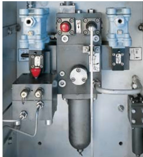
Shown with remote control 0 and SHUT-DOWN in case of line break including torque limitation
